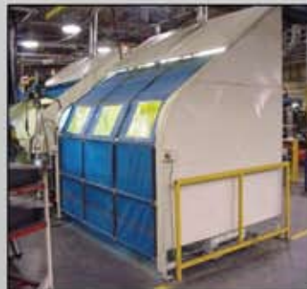
Protective Curtain Enclosures
